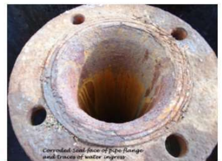
Figure 6 Traces of corrosion at seal face of flange (poor sealing caused water ingress)
