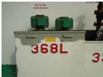
Figure 3 Vent head of the L.O. storage tank
