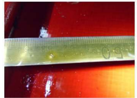
Figure 2 Sounding tape: Emulsified oil patches indicating presence of water
