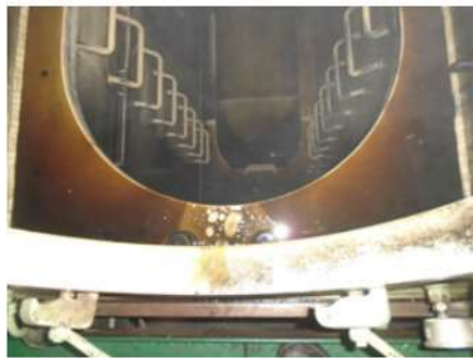
Figure 1 LO Sump: Emulsified oil patches indicating presence of water
